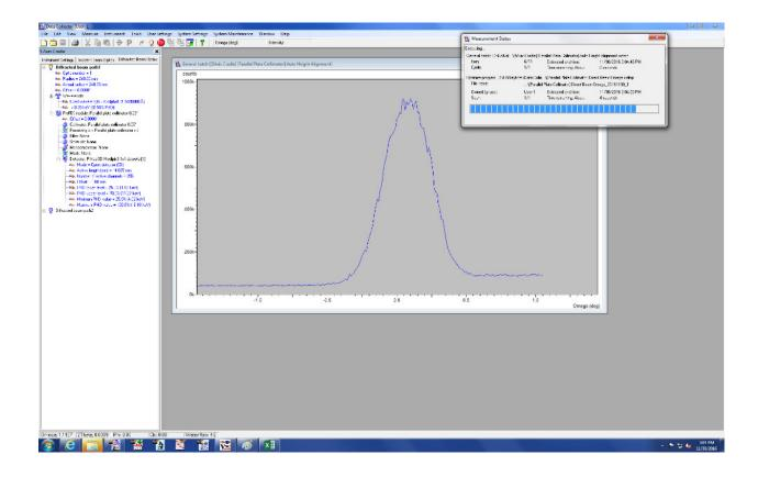
Towards the end of the automatic procedure, the routine will ask to remove the Cu attenuator and the Parallel Plate Collimator Slit. Replace the Cu attenuator by an appropriate mask (not wider than your sample) and remove the PCC slit.
