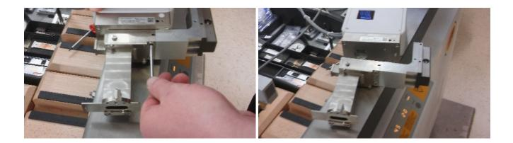
Take off the FASS holder and carefully place it in a save place inside the cabinet.
