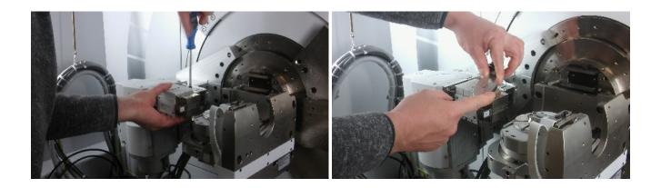
The detector cannot be remounted right away. It first has to be taken off the FASS mount and affixed to the PCC mount instead.
