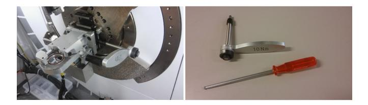
When the screw is far enough out the stage can be lifted out of its holder (it is secured with two pins in the back). Hold the stage securely with two hands at the bulky metal frame (not at any fragile parts or electronics, and do not grab into the central sample holder area). Turn it towards you and up, and lift it out until the pins are completely off the sample stage mount. Place it carefully into a save corner inside the instrument housing. Do not disconnect any of its cables.
