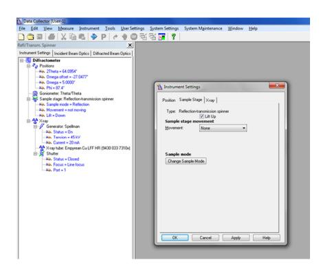
Check "Lift up", Click "OK" to move the lift up again prior to changing the stage and close the pop-up window.
