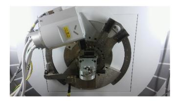
When prompted by the on screen messages remove the reflection transmission spinner stage.
