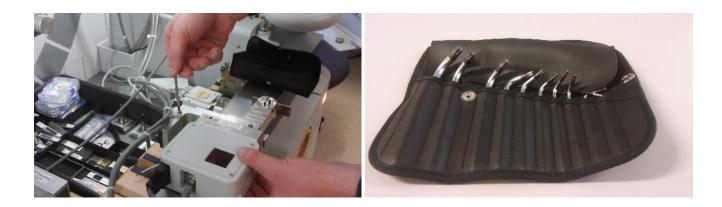
The detector is mounted to the FASS holder with two hex mounting screws and one pin. Loosen the screws completely. Use the T20 hex Ellen wrench from the black pouch inside the cabinet for this. The screws will remain with the FASS holder.
