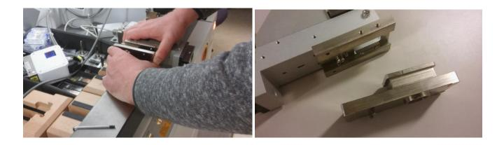
Mount the slid off holder onto the detector using its two hex mounting screws and the pin. Slide the mount and detector back onto the PCC holder.
