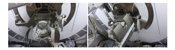
Connect the stage cable to any of the five slots to the right of the cabinet (look for red dots for cable plug orientation).
